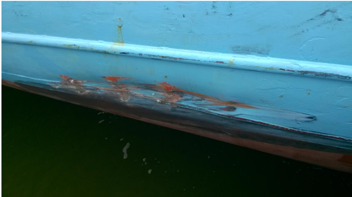
Photograph 3. Dent in plating of Bomar Victory where it collided with Virtus
