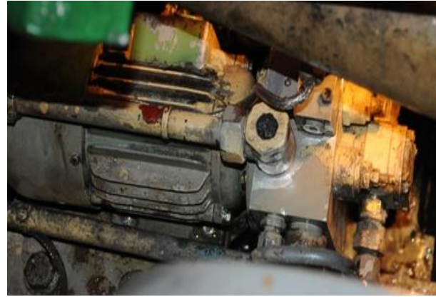
Photograph 3: Oil pressure pump of the adjustable propeller hub driven by means of an electric motor
