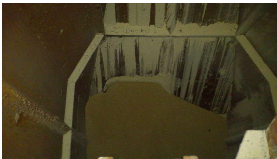
Photograph 5. Entrance to the hold no 7 covered with cargo - view from the inside of the ladder way
