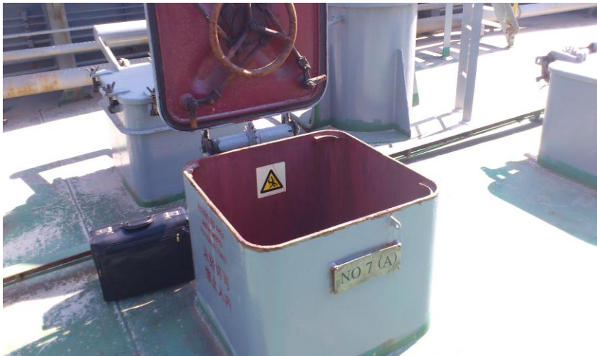
Photograph 4. Entrance to the ladder way to the hold no 7
