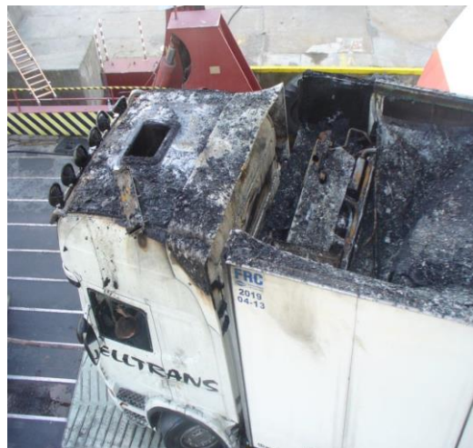
Photograph 6: The car, whose cooling unit was the source of fire on „Stena Spirit” (WIM 60/16)
