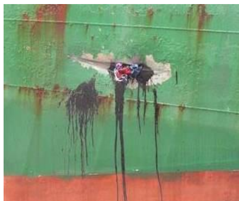
Photograph 12: Damaged (pierced) sheathing of the hull of "Green Egersund" (WIM 39/15)
