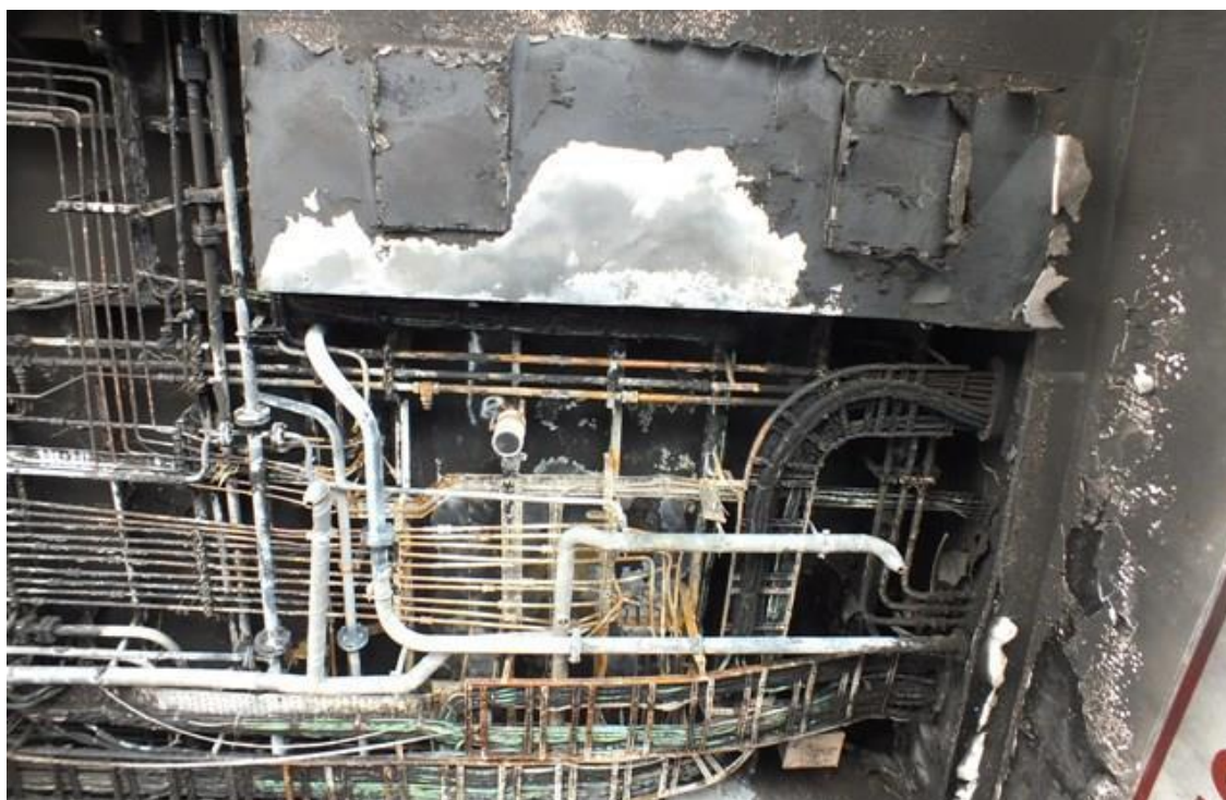
Photograph 7: Hydraulic installation damaged during fire on „Stena Spirit” (WIM 60/16)
