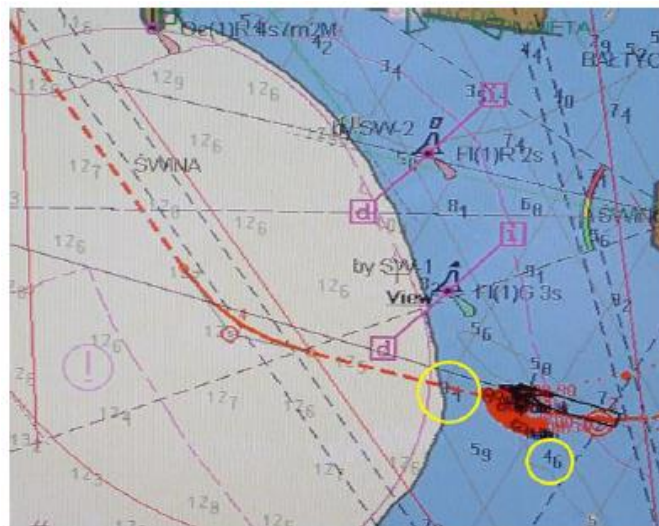
Figure 2 Screenshot of the ECDIS on Peak Bergen with the planned voyage route with an indication of the current depths of the water.
