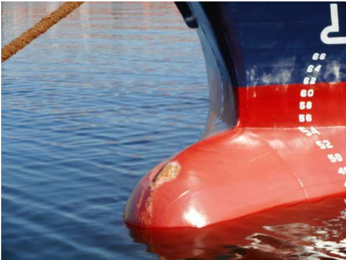
Photograph 2: Damage of the bulbous bow visible on the exterior
