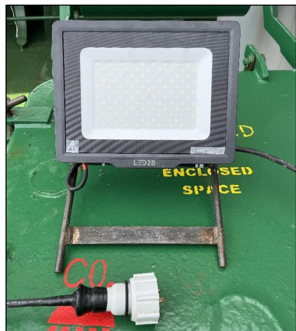
Figure 3: A portable cargo hold light used on board
