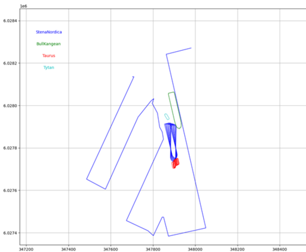
Figure 5 – Reconstruction of the SN towing set passage using combined AIS and VDR information of SN movement for stage 3 (UTM system, grid every 200m).
