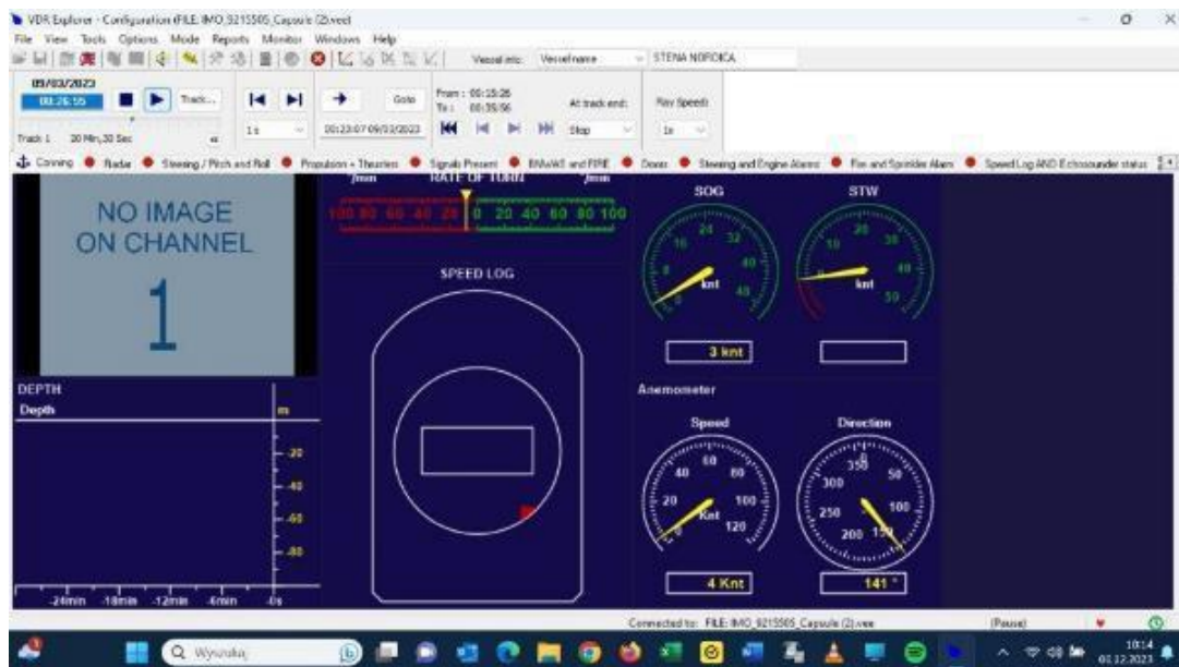
Photo 10 – Speed of the ship 'Stena Nordica' as read from the VDR recording at the time of collision.
