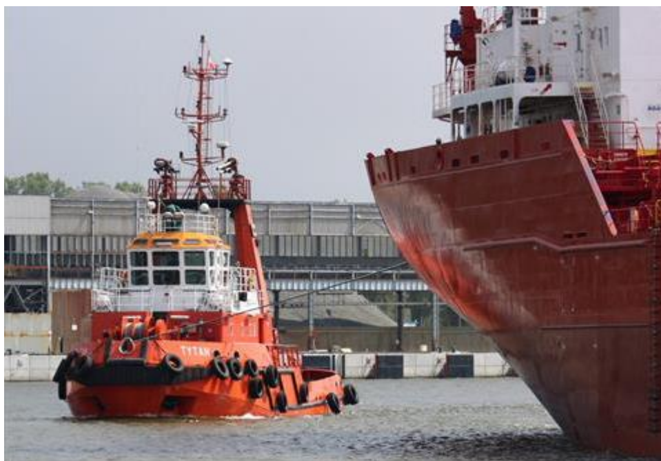
Photo 7 – 'Titan' working as an in-direct assist tug on the aft and its towing equipment in the form of a bow fairlead ( www.wobiektywieshipspottera.blogspot.com , by W. Danielewicz).
