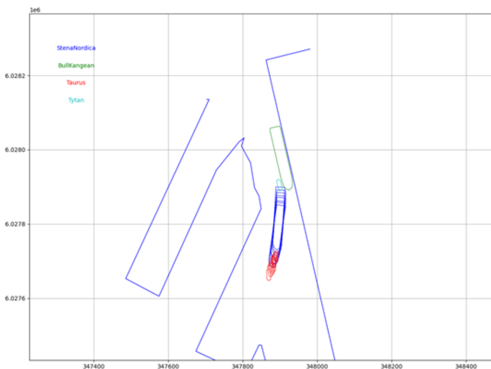
Figure 4 – Reconstruction of the SN towing set passage using combined AIS and VDR information of SN movement for stage 2 (UTM system, grid every 200m).
