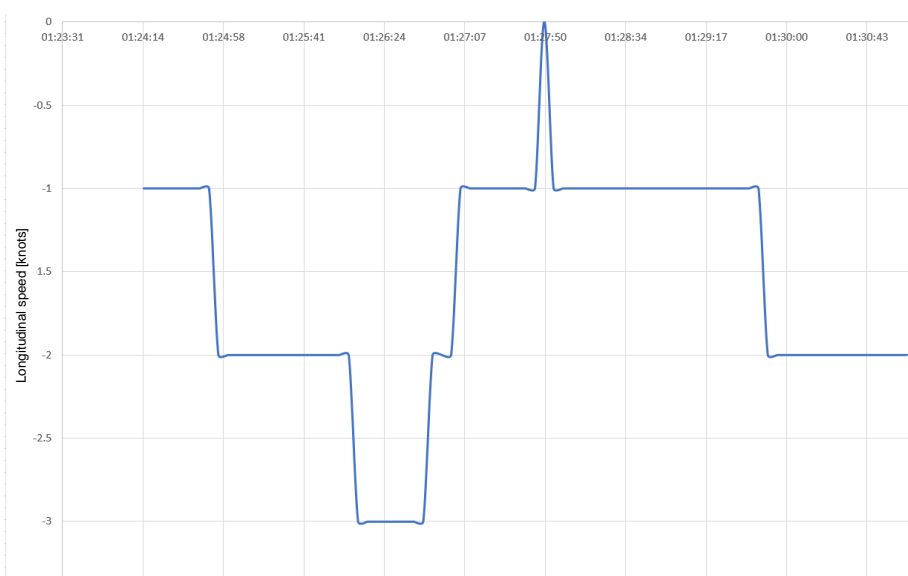
Figure 16 – Ferry longitudinal speed in knots based on log record from VDR (GMT time).
