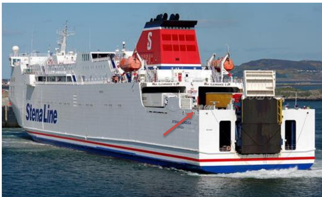
Photo 5 – Fairleads arrangement and stern ramp, view on the PS aft of the 'Stena Nordica' (www.shipspotting.com, by Willie Ryan) – before rebuilding i.e., without the so-called Duck Tail on the stern.
