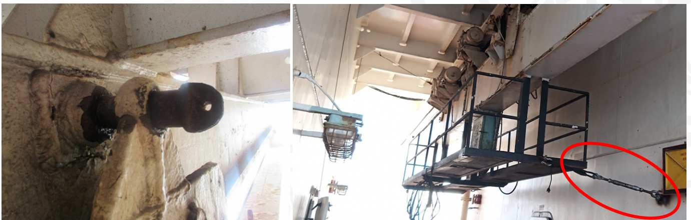
Sistership arrangement: securing pin (original design) and retrofitted securing arrangements (ringed)
