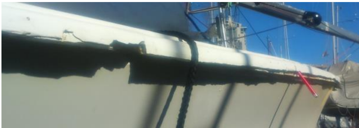
Photo 5 – damage to the deck-board junction
