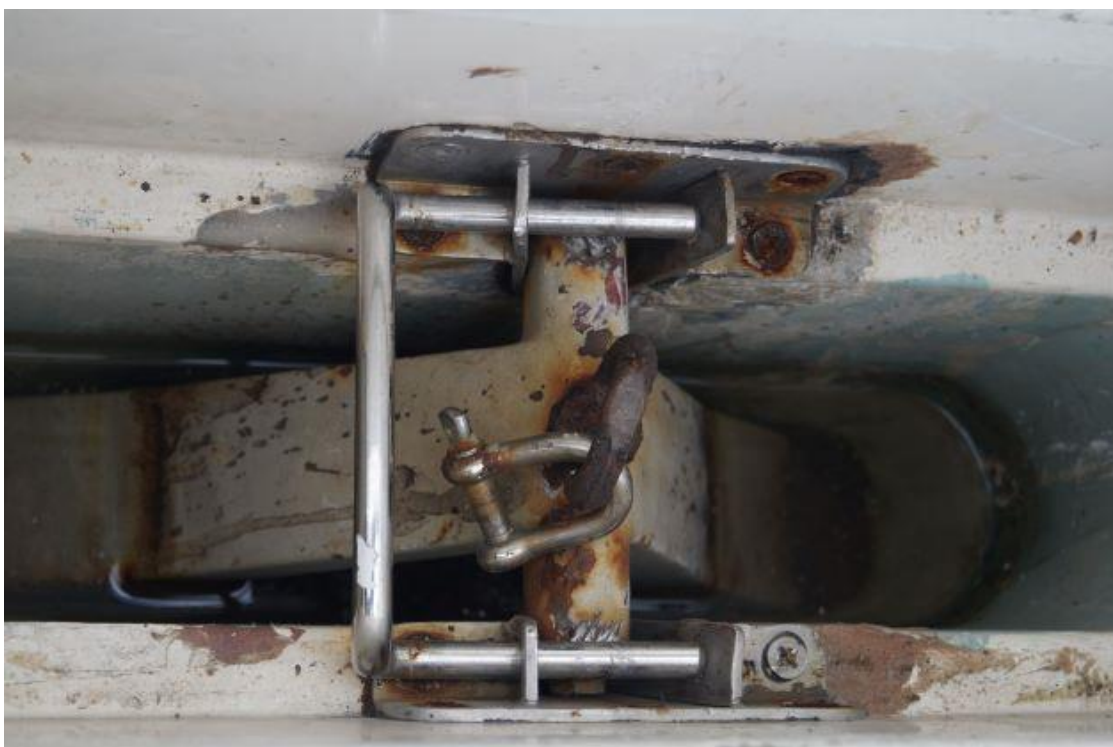
Photo 9 – the holes in the centreboard locking seat are not aligned and do not allow the ballast fin to be properly secured.
