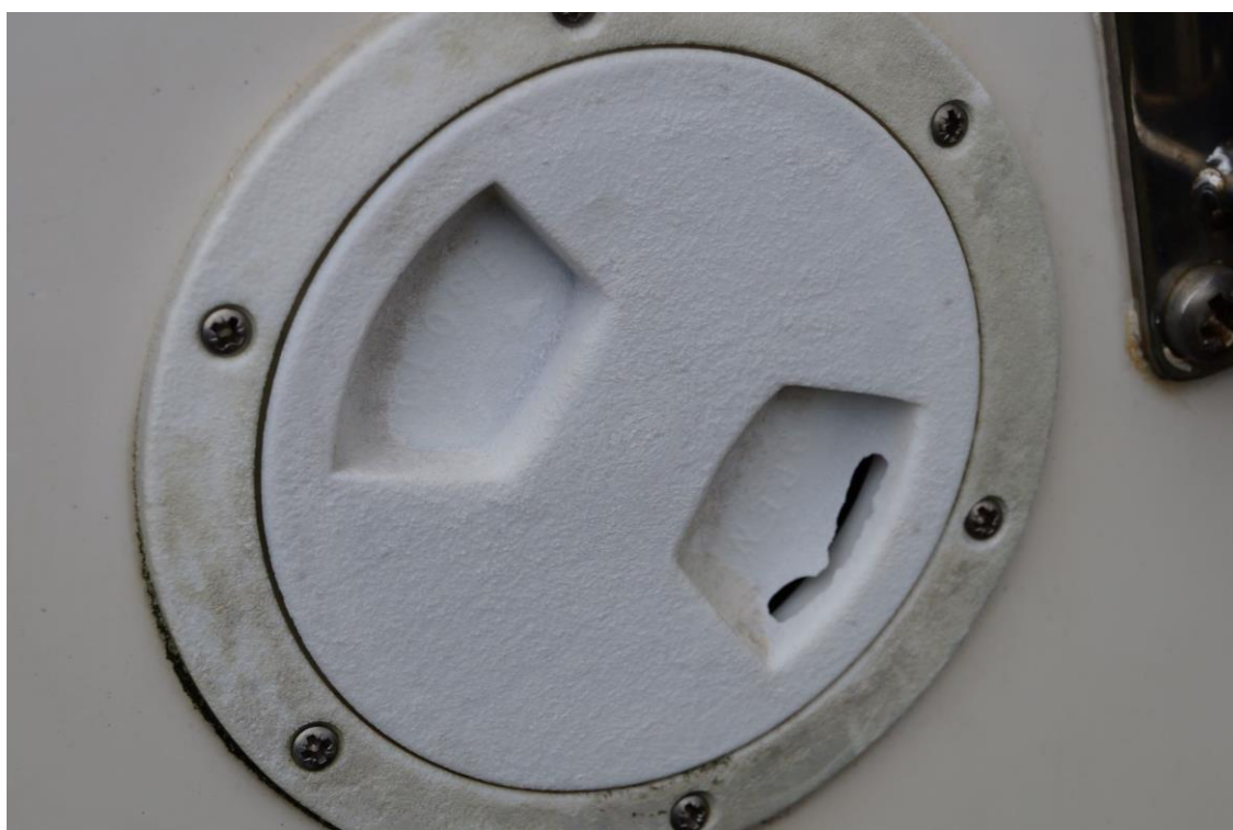
Photo 8 – damaged cap of the control hatch
