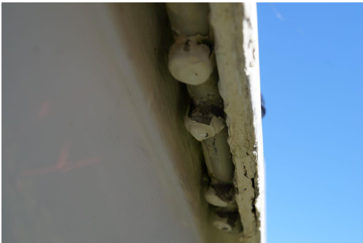
Photo 6 – damages to the shroud futtock
