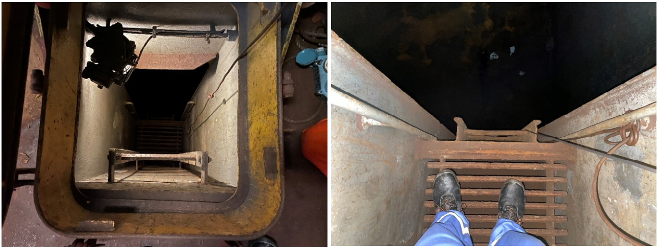
Access to hold 7, looking down from cross-deck tunnel and ladder platform, hatches closed
