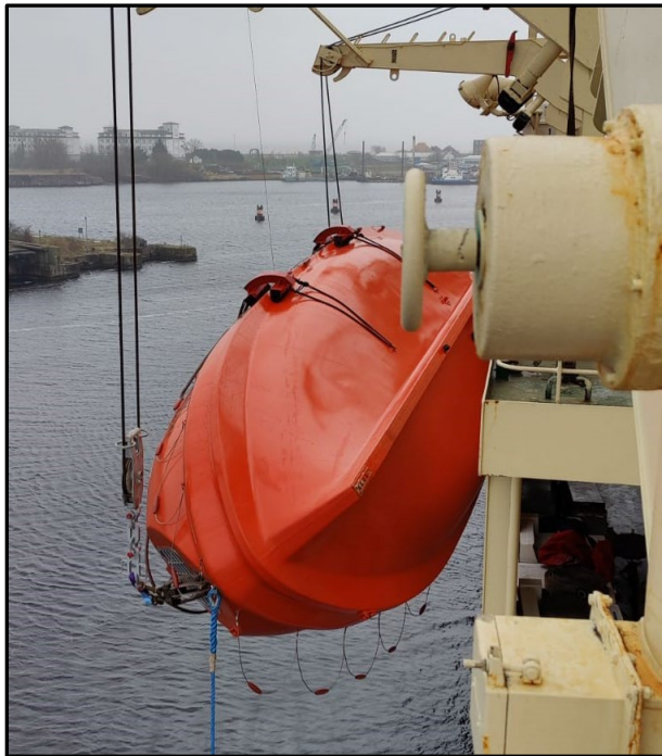
Figure 3 - Lifeboat listing more than 90 degrees w/ crew inside.
