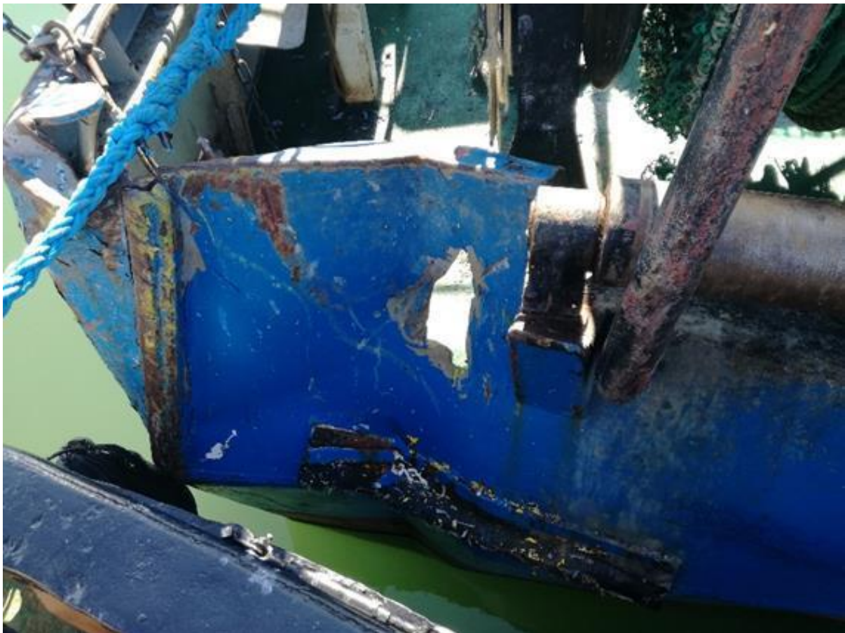
Photograph No. 4 Damage to the fishing cutter Ancilla WŁA-68
