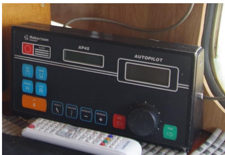
Photograph No. 6 Autopilot of fishing cutter UST-31
